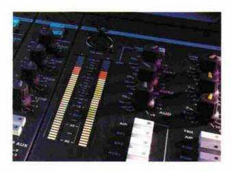
The LED-meter in de Master module shows the signal selected by the Multisource Selector. It can also be set to show the PGM output signal.
