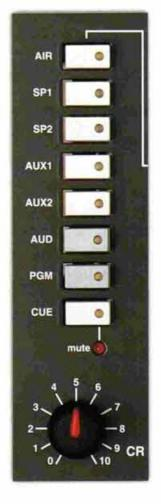
The Multisource Selector has automation capabilities enabling the engineer or presenter to concentrate on the actual program.
